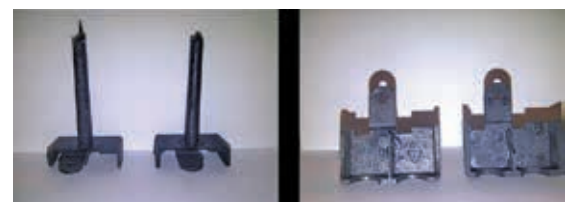
Figure 8. Printed mold components in Digital ABS. The metal sprue bushing will insert into the hole in the mold part on the far right.
