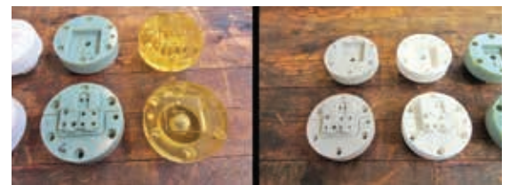
Figure 3. The 3D printed inserts include, on the left, Digital ABS (green) and Transparent (yellowish), and on the right, PA12 (with glass fiber, gray) and PA (without glass fiber, white).
