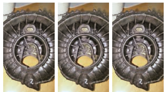
Figure 11. The injected part from the Transparent mold with the tears
