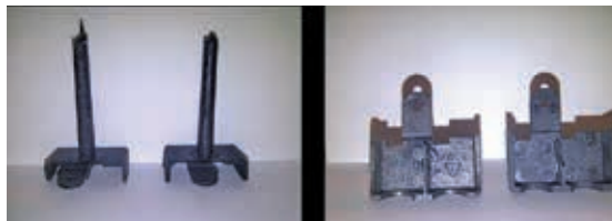
Figure 5. Injected cover cables prototype (left) and injected cover cables prototype, bottom view (right).
