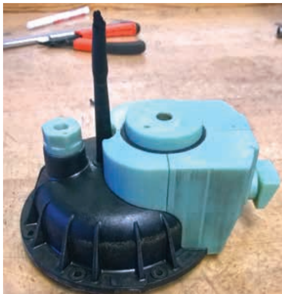
Figure 14. A side view of the injected part with attached molds part and sprue
