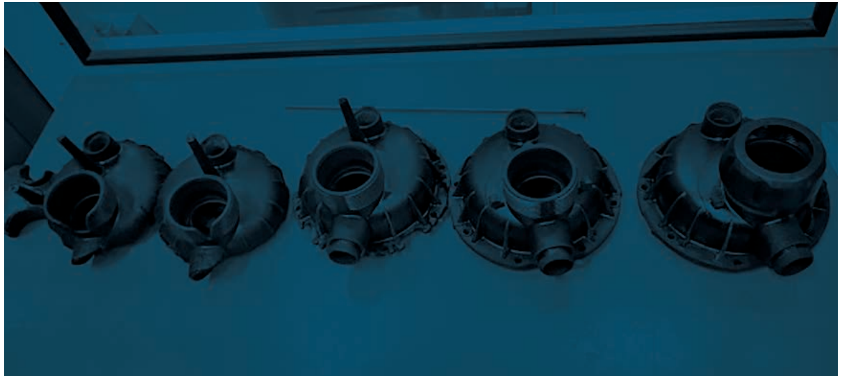
Figure 12. The first six parts using the Transparent mold.
