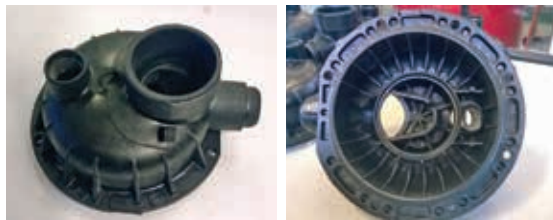
Figure 6. Top and back views of the part as it came out of the printed core and cavity. Notice the complex ribbed sections in the right picture. The part's dimensions are 160 mm (diameter) and 70 mm (height).
