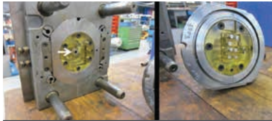
Figure 4. Cavity and core side of the mold. The arrow indicates the sprue bushing, an important design feature.
