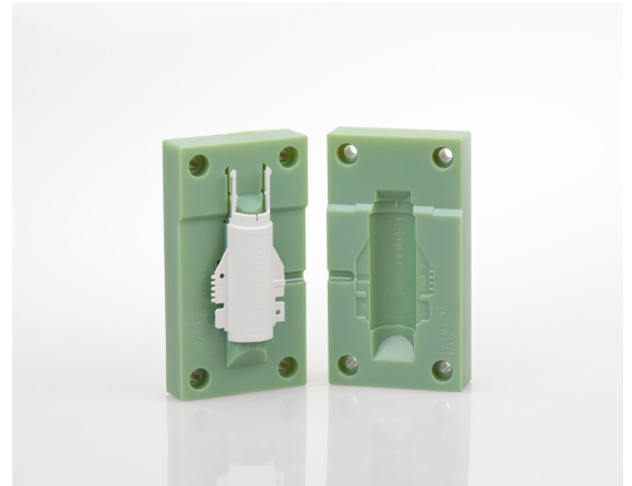
Figure 7: Digital ABS Plus on the Connex3 builds tough injection molds fast for Turck.
