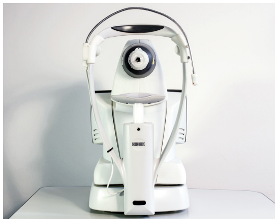
Figure 3: The external case of Nidek's prototype Gonioscope® was built on a Connex3 3D Printer.
